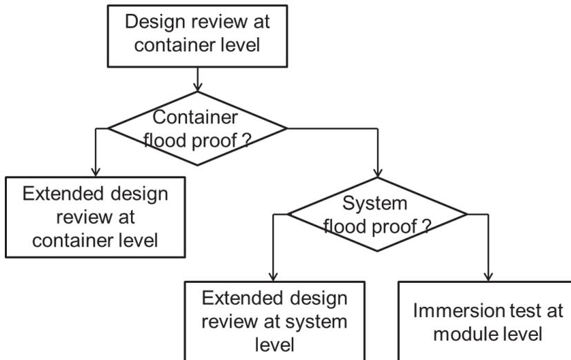
The first step in the procedure will be a design & construction review, depending on the specifications of the (sub)system manufacturers or the system integrator. The main barrier against flooding of the storage system is the container. Design and installation requirements are prescribed, to minimize the risk of flooding. It is recommended that the containerized storage system is placed in such a way that the probability of flooding is less than 1 in 1000 years.
