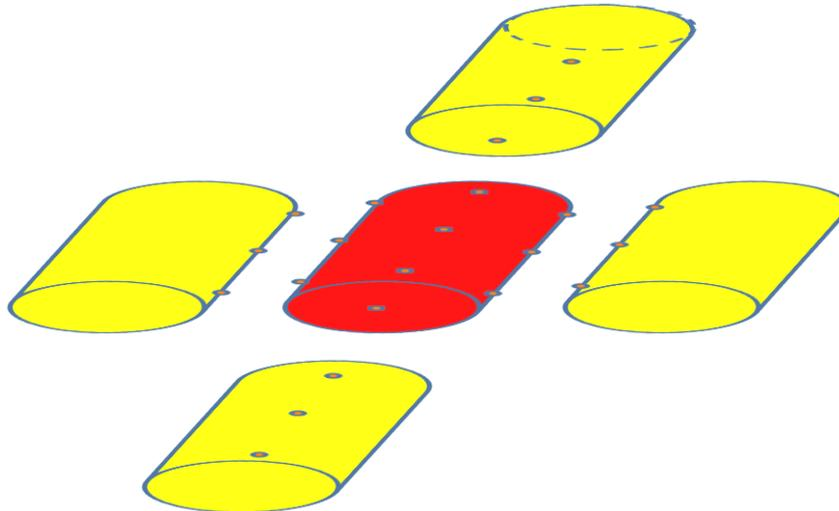
On a cylindrical cell to be treated (red) there shall be mounted 13 thermocouples to get a temperature distribution of the surface temperature of the cell. 12 thermocouples on the cylindrical surface, 4 mounted around the diameter and three of such “rings” distributed over the longitudinal axis. The thermocouple 13 will be located where the venting area is located.
