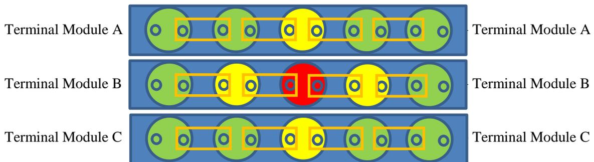
All dummy cells (green) are short circuited between its cell terminals to allow charging over the + and – terminals of the modules.
